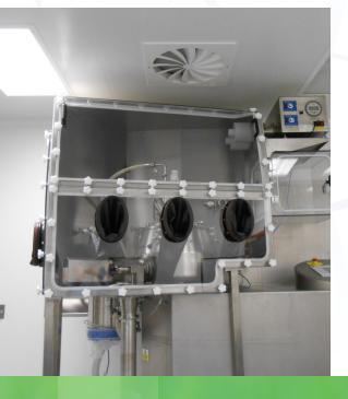
These products are fabricated and constructed by heat and high frequency electronic welding and computerised cutting systems, and have for many years been at the forefront of technology in flexible containment solutions for Semiconductor Clean room and Pharmaceutical applications where levels of containment below 1 micron per cubic metre are required.
