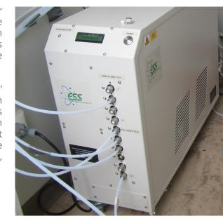
With a high sensitivity, membrane inlet giving a wide dynamic range from low ppb to percent levels, PharmaSys is the system of choice for accurate on line process control of VOC and solvent monitoring applications. The quality of the data means that it can be used in six-sigma modelling in generating process quality improvements.
